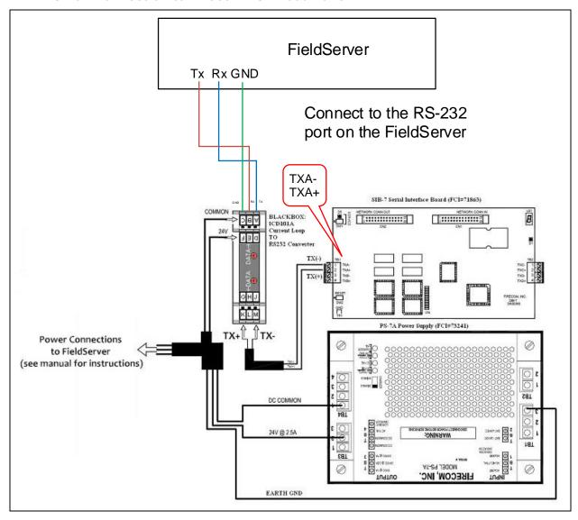
The FieldServer is connected to the Firecom panel via the sib-4 serial interface board port a, b, c or d. The port must be configured as Firecom ASCII protocol in the Firecom ISN 2000 data entry program.
